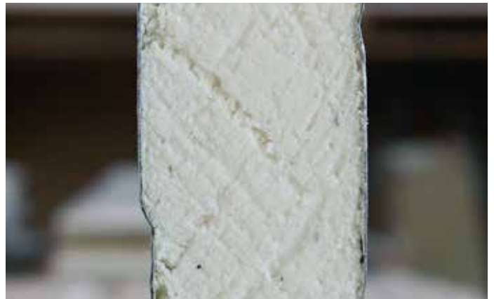
Flame-retardant PUR panels (building material class B)
