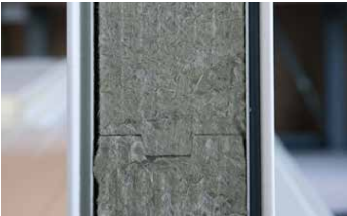
Non-combustible mineral wool panels (building material class A)
