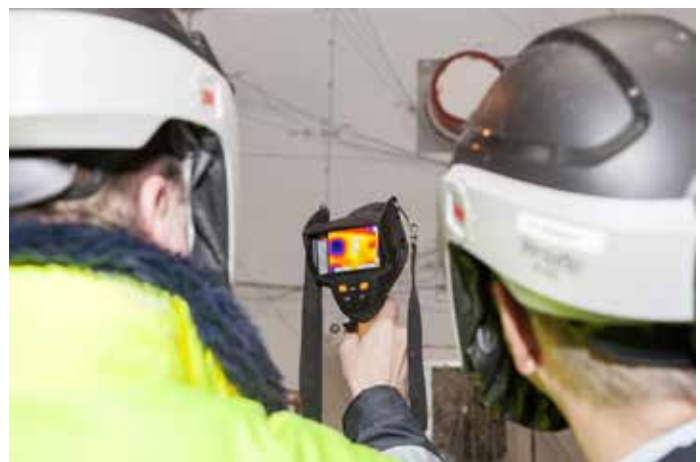
Checking fire tests with thermography
