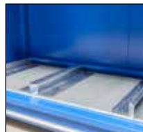
"Pushback trolley" - system for "Last-In-First-Out" loading
