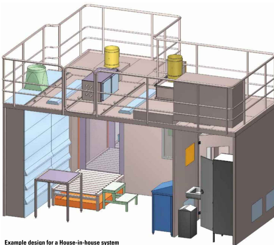
Example design for a House-in-house system
