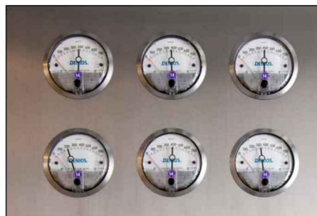
Monitoring of differential pressures, air speed and air quality, analogue or digital
