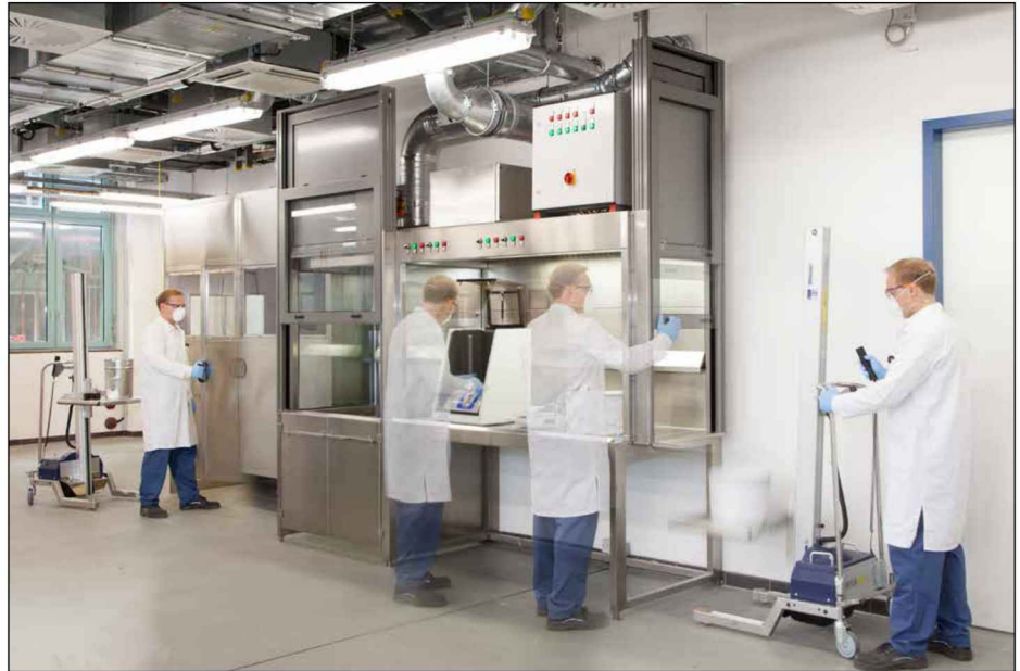
The intensive mixer is housed in a free workstation with wing doors, which increases employee safety and also reduces the noise level of the mixer.
