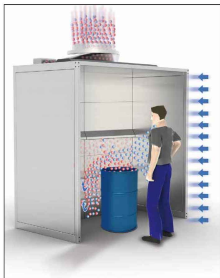
Premium free workstation functional drawing
