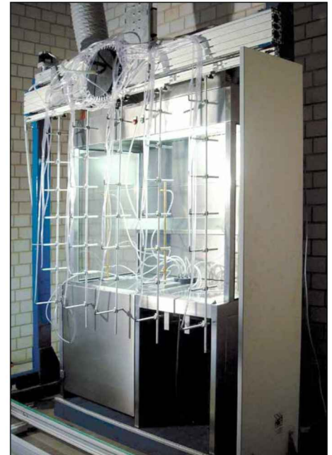
VARIO Flow work bench (Premium model) in test set-up for determining retention capacity
