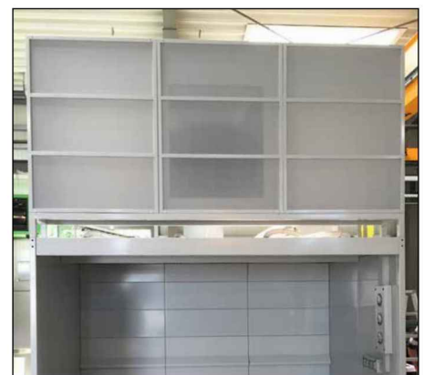
Air recirculation plenum for returning filtered air to the room
