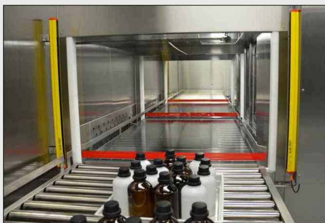
Material air lock with spray drying system for IPA disinfection
