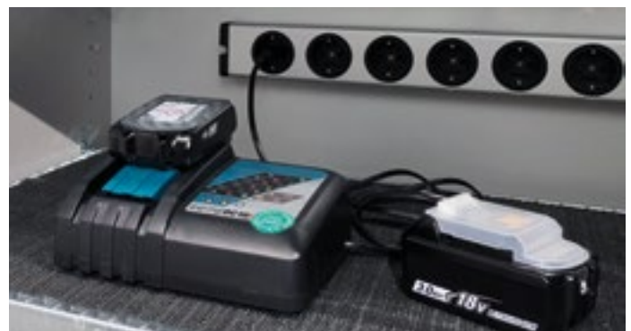
Charging station in safety cabinet
